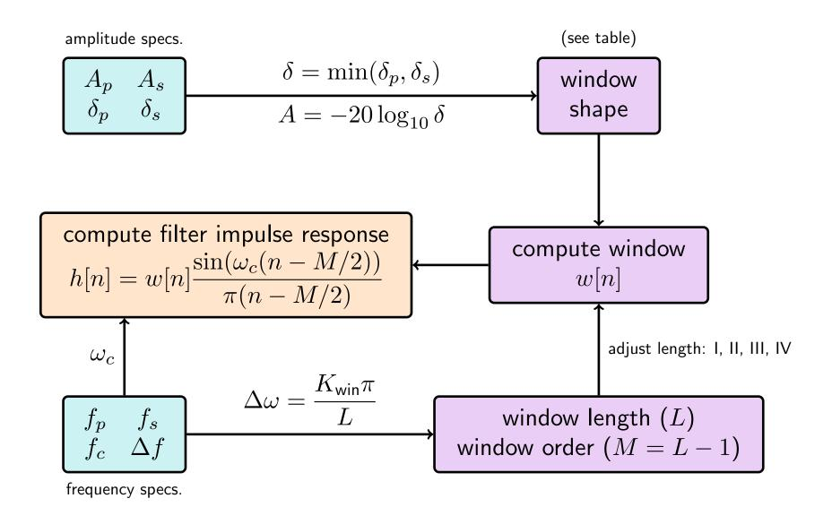
Does the filter meet the specifications? Check |H(f)|. If not, increase length and check again.
