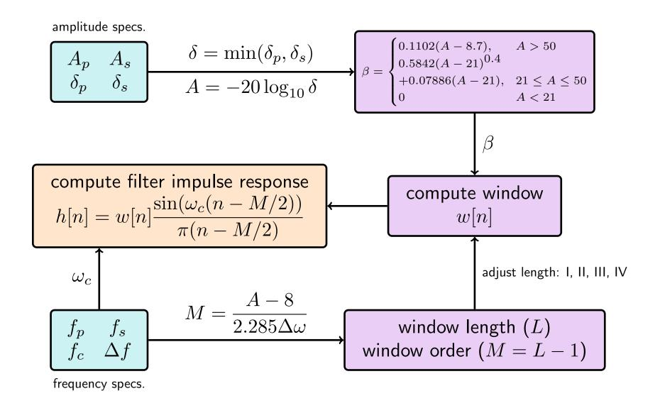
Does the filter meet the specifications? Check |H(f)|. If not, increase length and check again.
