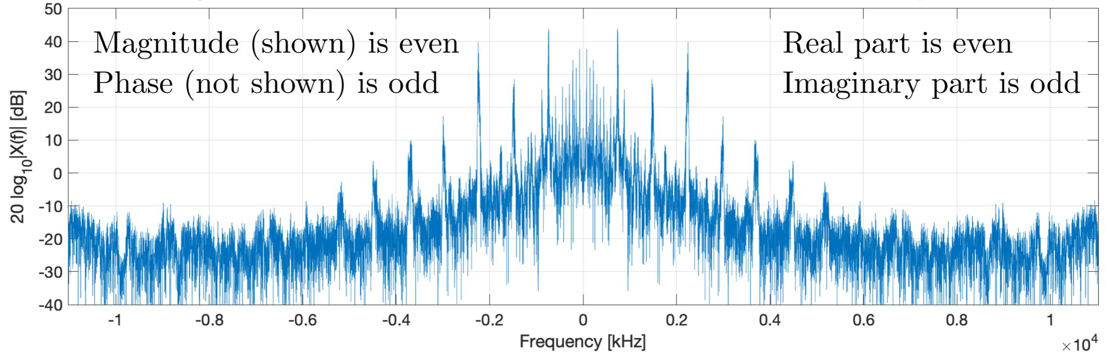
Radio signal is complex, spectrum exhibits no symmetry
