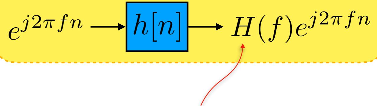
$H(f)$  gives the response of the system when the input is an everlasting complex exponential at frequency  $f$ .
