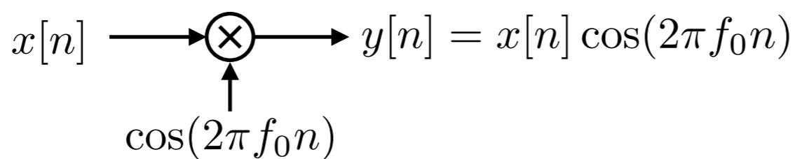
Bandwidth of modulated signal is twice the bandwidth of the baseband signal.
