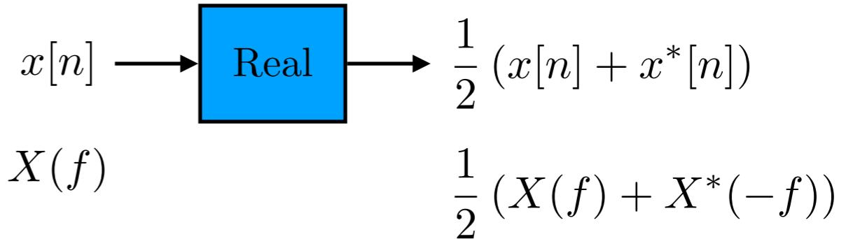
Taking the real part in the time domain of a complex signal produces the Hermitian part in the frequency domain.
